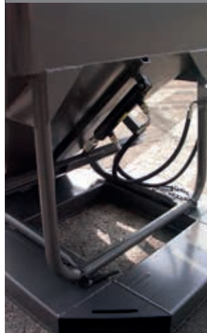
HYDRAULIC OPENING OF THE BUCKET
