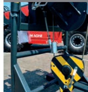
HYDRAULIC ASCENT AND DESCENT LIMIT STOPS
