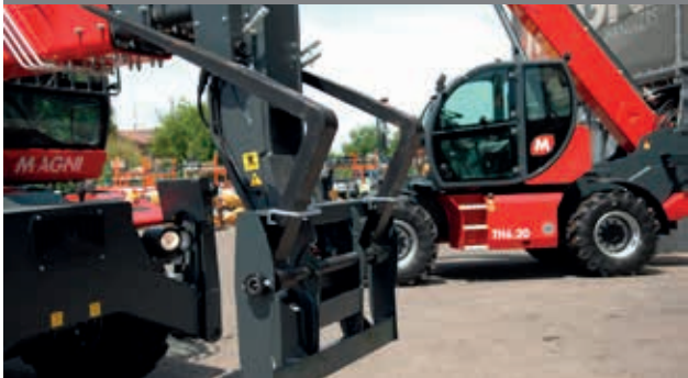
FOLDED FORKS FOR ROAD CIRCULATION
