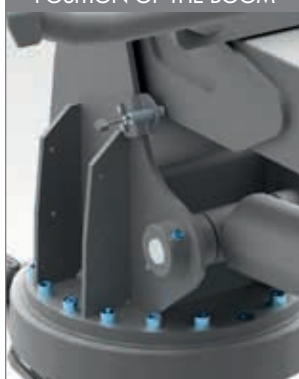
SENSOR FOR DETECTION OF THE POSITION OF THE BOOM
