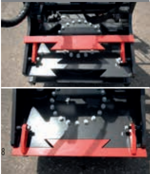
EQUIPPED WITH ROTATION BLOCKING BAR +/- 90°
